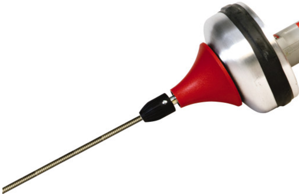
Fig. 2 Push Cable Into Drum
