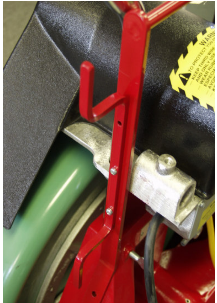
Move to Right hand side and repeat Bracket drilling and bolting.
