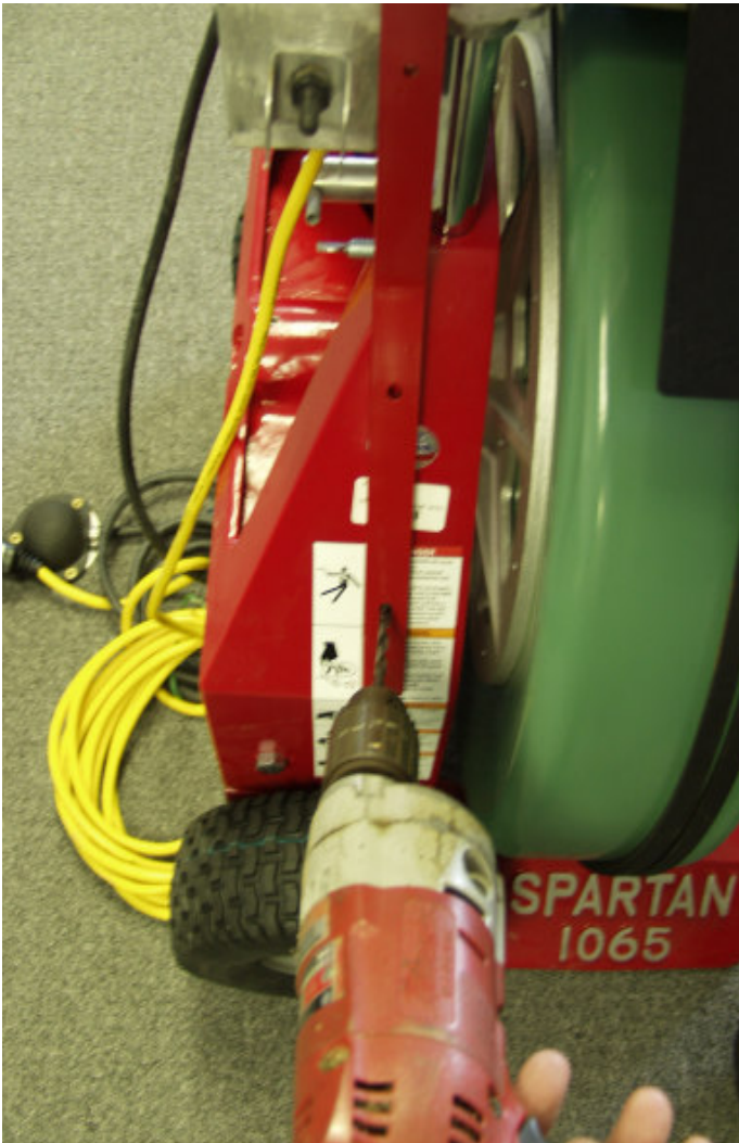
Finish by relocating the Cord Wrap Bracket drilling and bolting.
